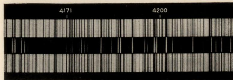
length  $BX$ , the greater will be the distance  $EK$ , and from the distance  $EK$  and the distance of the screen from the grating it is easy to calculate the wave-length.
