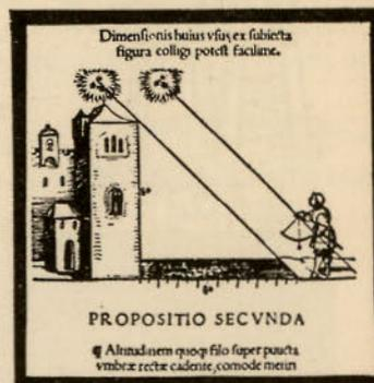
FIG. 7. USING A SMALL QUADRANT
